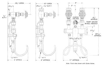
NOTE: A strainer and steam trap is recommended to be used in conjunction with all our steam mixing units. Foreign deposits in supply lines can effect ball check durability. Proper steam and water treatment is recommended to ensure proper performance and durability. Unit should be shut-off when not in use for extended periods of time.
