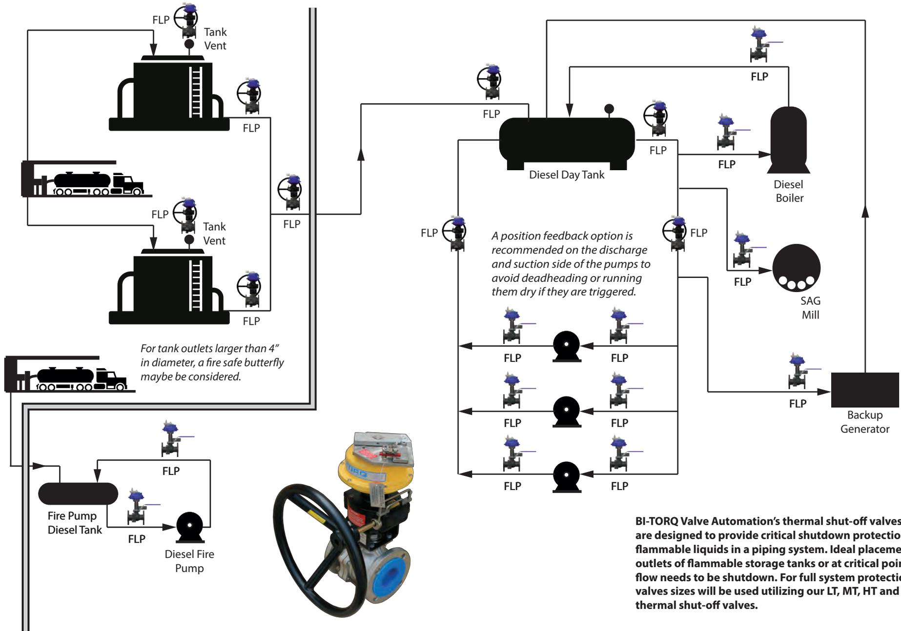
BI-TORQ Valve Automation's thermal shut-off valves (FLP series) are designed to provide critical shutdown protection on flammable liquids in a piping system. Ideal placement is on the outlets of flammable storage tanks or at critical point in a where flow needs to be shutdown. For full system protection, a variety of valves sizes will be used utilizing our LT, MT, HT and BT series thermal shut-off valves.
