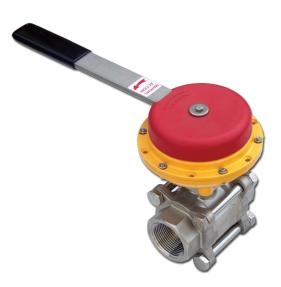
Spring return "deadman" handles will help you meet OSHA requirements or plant specifications where a valve must return to the closed position after operation. Unlike a standard lever handle or gear operator which will remain in the last position, our assemblies ensure that the handle will always spring return to its original, pre-designated starting position.
