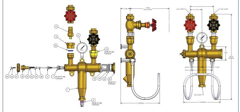
NOTE: A strainer and steam trap is recommended to be used in conjunction with all our steam mixing units. Foreign deposits in supply lines can effect ball check durabilility. Proper steam and water treament is recommended to ensure proper performance and durability. Unit should be shut-off when not in use for extended periods of time.
