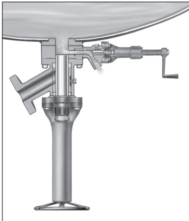
Fig. 2 - Drain Valve Open for Sample
